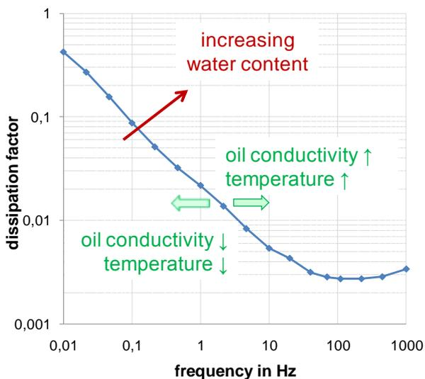
**Figure 5:** Main influences on measured dielectric response curves
