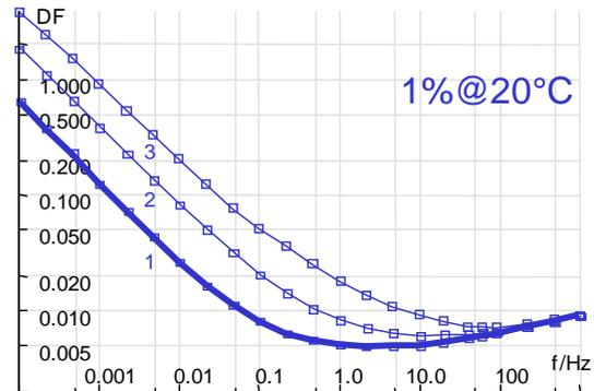
**Figure 2:** Dielectric response of cellulosic material at 20°C with 1% (2% and 3%) water content
