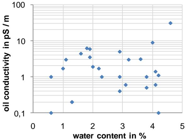
**Figure 10:** Oil conductivity and water content for various instrument transformers of different condition
