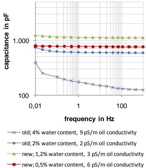
**Figure 11:** Frequency dependent capacitances of various instrument transformers depending on frequency
