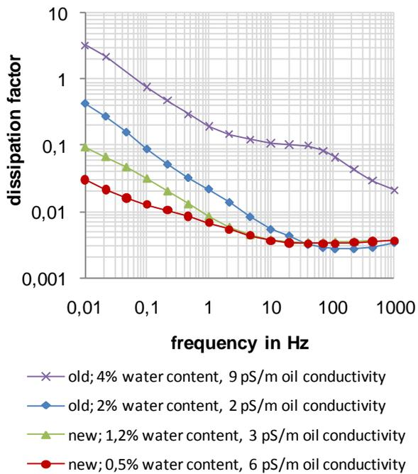
**Figure 4:** Dielectric response of instrument transformers of different age and condition
