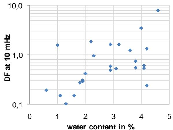
**Figure 9:** Dissipation factor at 10 mHz and water content for various instrument transformers of different condition
