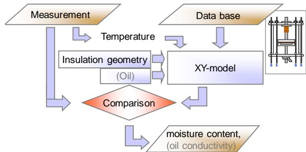
**Figure 6:** Calculation of the water content based on comparison of the measured dielectric response to a modelled curve
