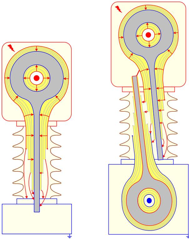
**Figure 7:** Schematic drawing of the insulation inside a CVT (left) and a CT (right), the losses (current flow through the insulation) are marked with arrows
