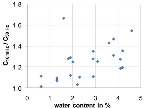
**Figure 12:** Ratio of capacitance values between 10 mHz and 50 Hz
