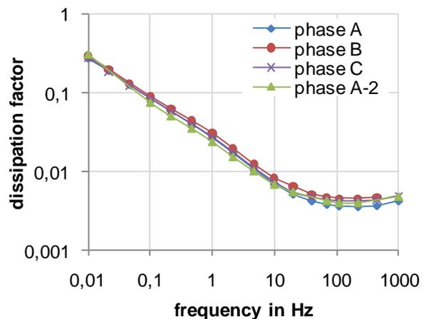
**Figure 3:** Dielectric response four current transformers of the same type, manufactured in 1963 (110N / 260kV), having a water content of 1.8 – 1.9% and an oil conductivity of 3 – 6 pS/m
