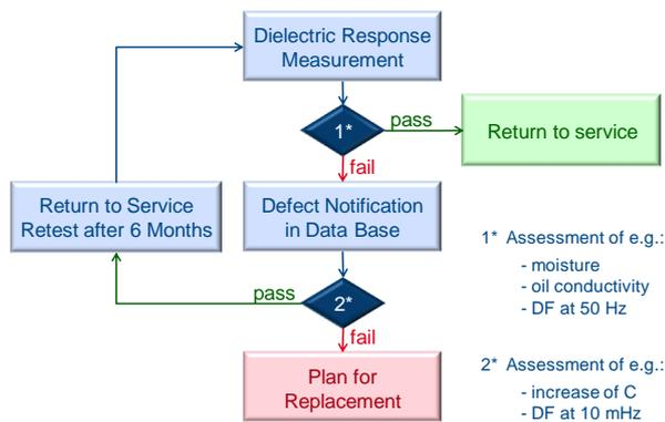
**Figure 13:** Example for a decision tree based on the results of the dielectric response
