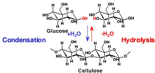
**Figure 1:** Schematic drawing of hydrolysis in cellulosic materials
