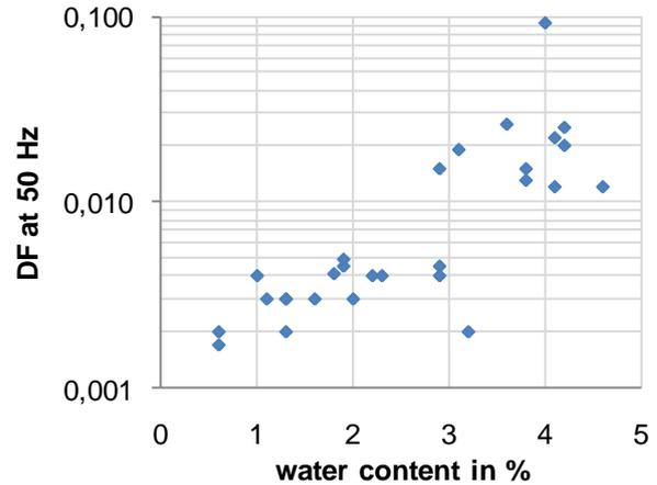
**Figure 8:** Dissipation factor at 50 Hz and water content for various instrument transformers of different condition
