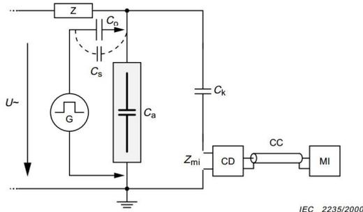
Fig. 4 Calibration according to IEC 60270 (general)
