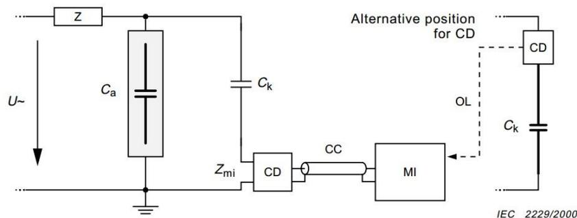
*Fig. 3 Test circuit for partial discharge measurement according to IEC 60270*
