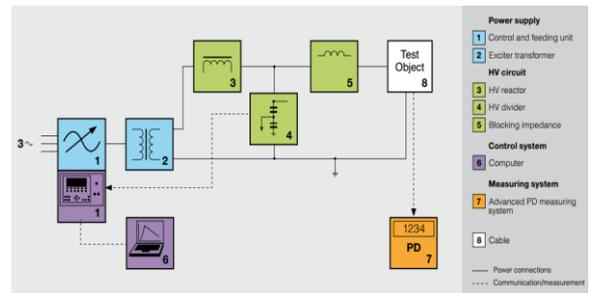
*Fig. 2 Block diagram of AC resonant test system for cable testing*
