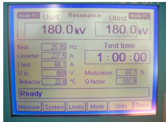
**Fig. 27** Screen of the operation unit of the resonance test set.
