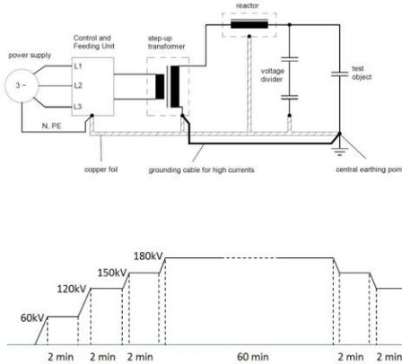
**Fig. 26** Scheme of the resonance test set and profile of the test voltage levels
