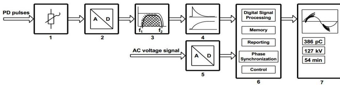
a) Direct A/D conversion of the input PD pulses
