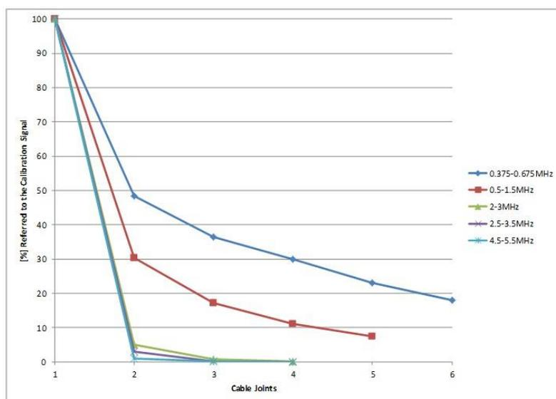
**Fig. 15** Damping of PD impulses along a cable for different measurement frequencies
