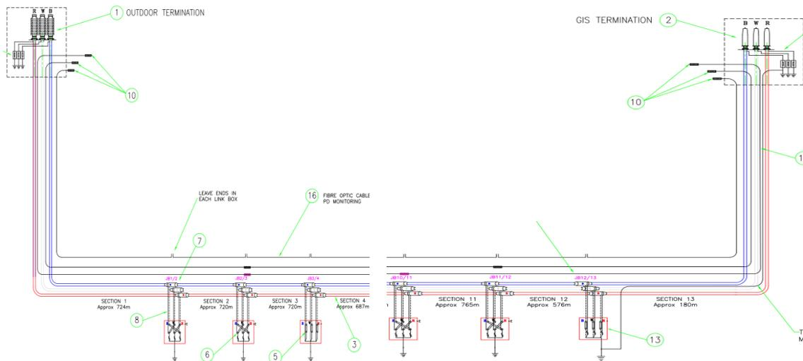
**Fig. 7** Typical cable scheme with link boxes for cross-bonding (6) and earthing (5 and 13)
