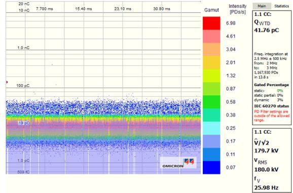
Fig. 29 PD measurement at the coupling capacitor with gating
