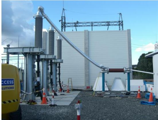
*Fig. 18 Outdoor termination with the HV test setup*
