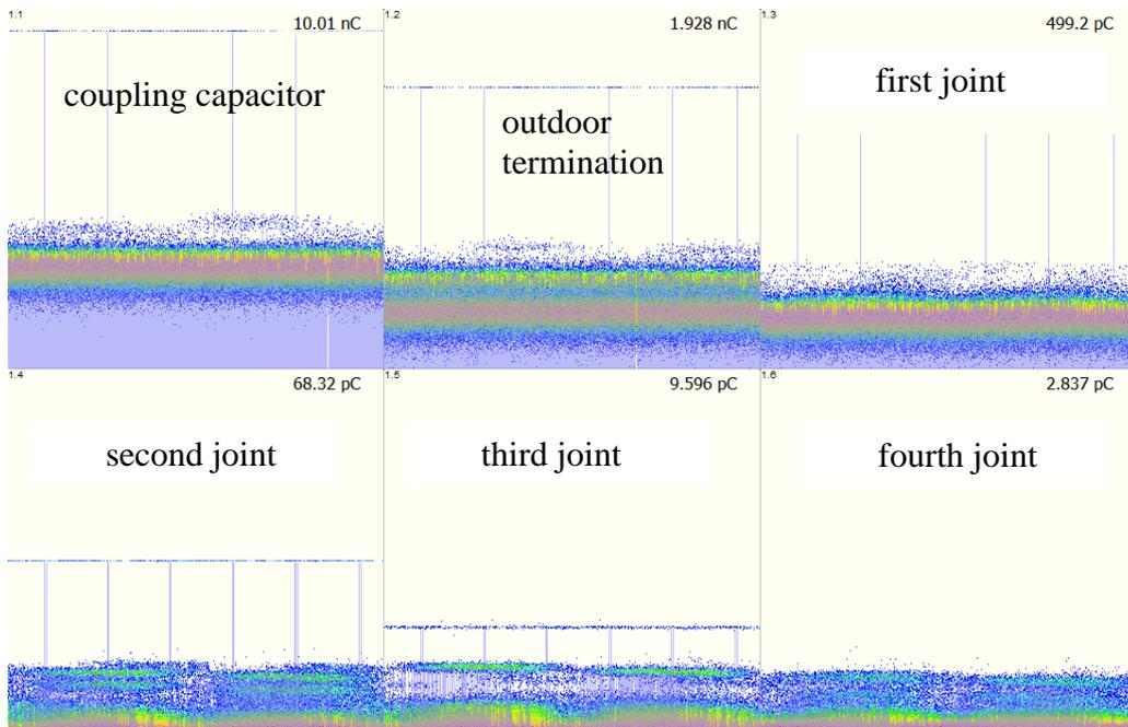
**Fig. 14** 10nC at the coupling capacitor yellow phase
