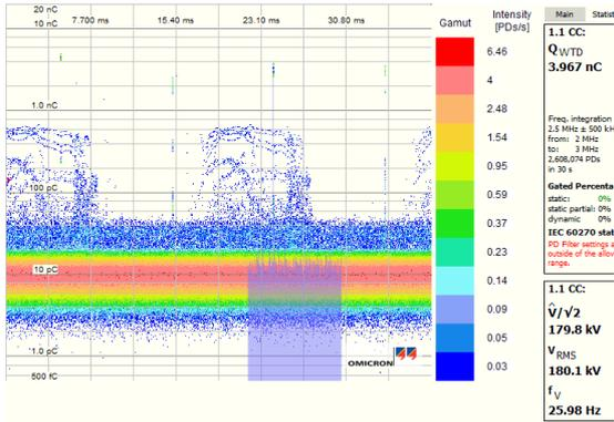
Fig. 28 PD measurement at the coupling capacitor without gating
