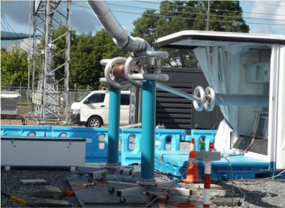
*Fig. 17 HV resonance test set with voltage divider, blocking impedance and coupling capacitor for PD measurement*
