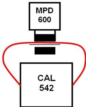
*Fig. 11 Performance check of HFCT's (principle)*
