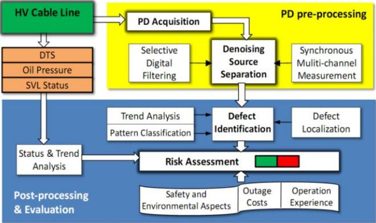
Fig.33 Concept of a cable PD monitoring system
