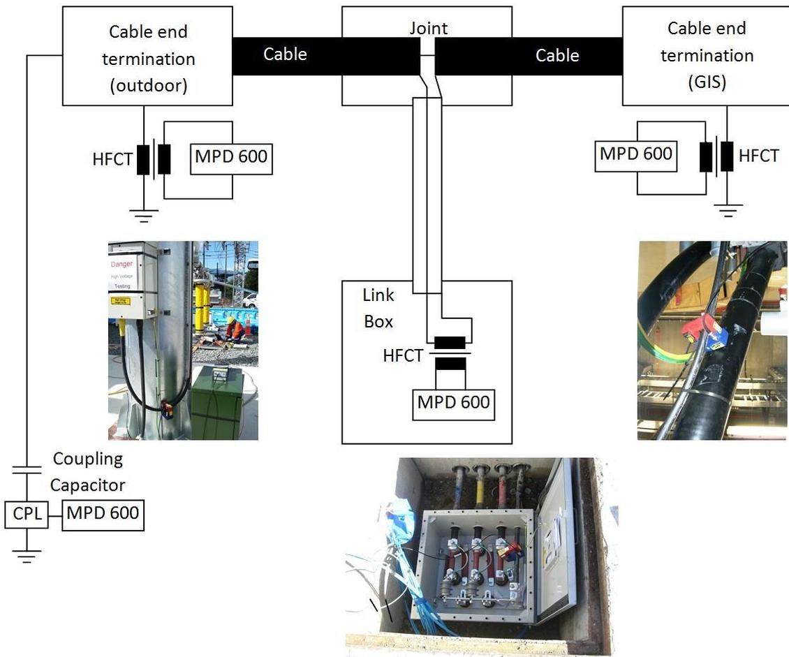
*Fig. 10 Test arrangement with MPD600 units at the coupling capacitor, the terminations and the joints*
