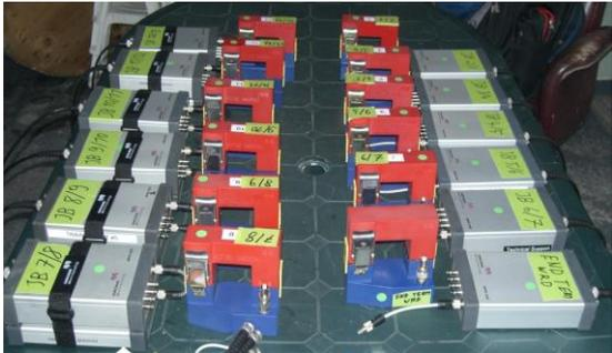
*Fig. 16 Preparation of the MPD600 with batteries and HFCT’s. The HFCT’s were equipped with an air gap in the core to prevent core saturation*
