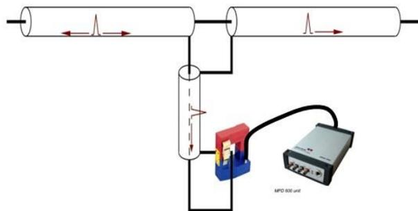
**Fig. 9** Measurement principle with HFCT in the link box
