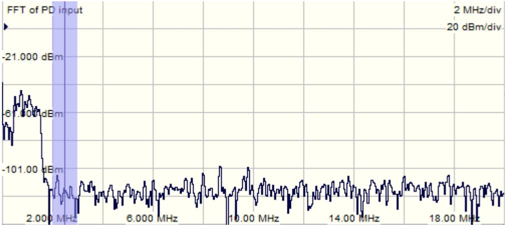
Fig. 13 Spectrum of external interference at a joint
