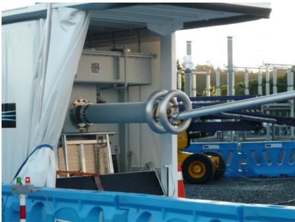
*Fig. 1 Resonance system for after-laying tests on cables*
