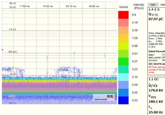
Fig. 30 PD measurement at joint two without gating
