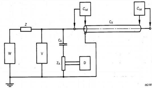
Fig. 5 Calibration according to IEC 60885 (cables)
