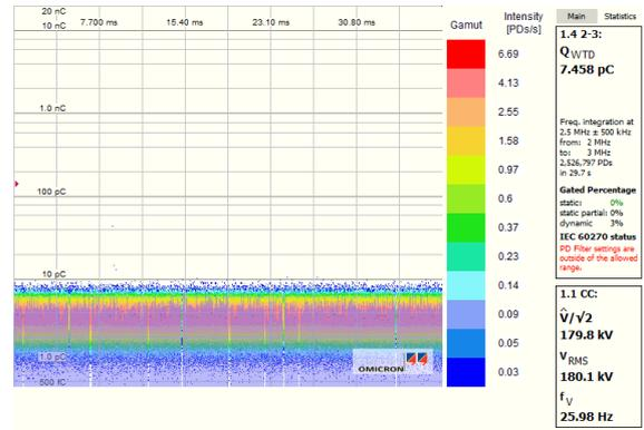
Fig. 31 PD measurement at joint two with gating
