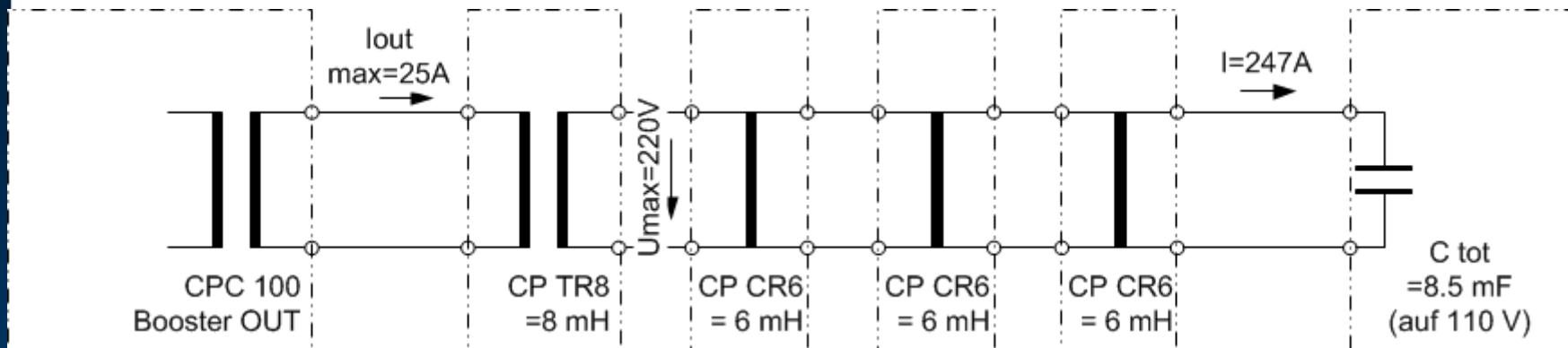
$$C_{110\text{ V}} = \frac{C_{\text{tot}}}{u^2} = \frac{1750^{-12}}{(242 / 0.11)^2} = 8.5\text{ mF}$$
