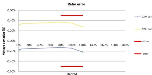
Fig. 15. Voltage ratio error at 100% and 25% of rated load
