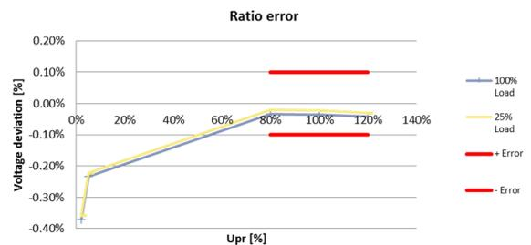
Fig. 10. Voltage ratio error diagram
