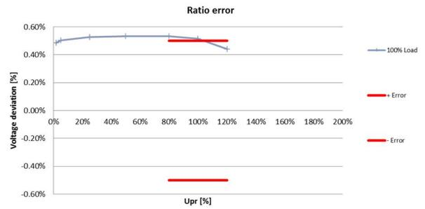
Fig. 14. Voltage ratio error at operating load (0.02VA) conditions
