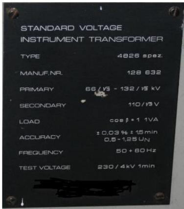
Fig. 1. Nameplate of reference VT
