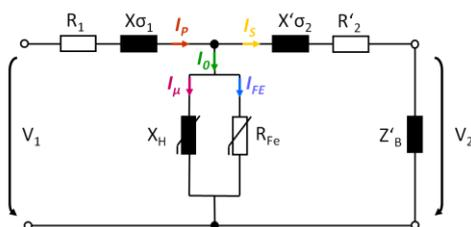
Figure 2: Equivalent circuit diagram of an instrument voltage transformer
