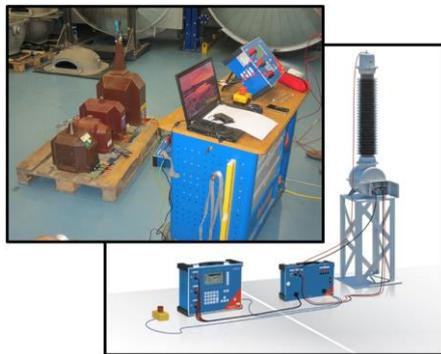
Figure 4: Test setup “model-based-calibration” with OMICRONs VOTANO 100
