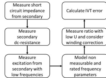
Figure 3: Methodology of the model-based method
