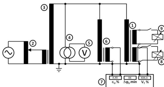
Figure 5: Test setup for accuracy measurement on IVT's
