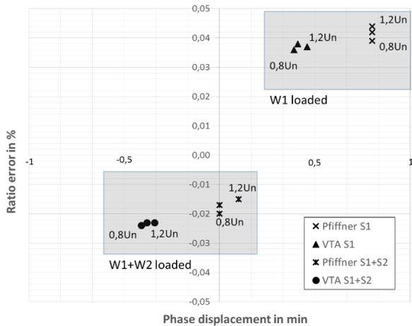
Figure 7: Measurement results of DUT 1 for different load condition of the two secondary windings
