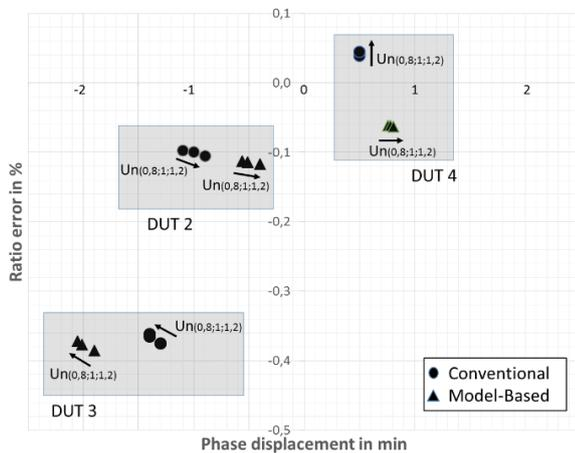
Figure 8: Measurement results of DUT 2 - DUT 4
