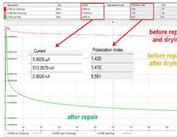
Figure 25 Polarisation current before and after repair
