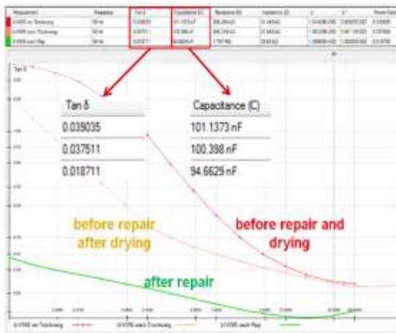
Figure 24 FDS before and after repair
